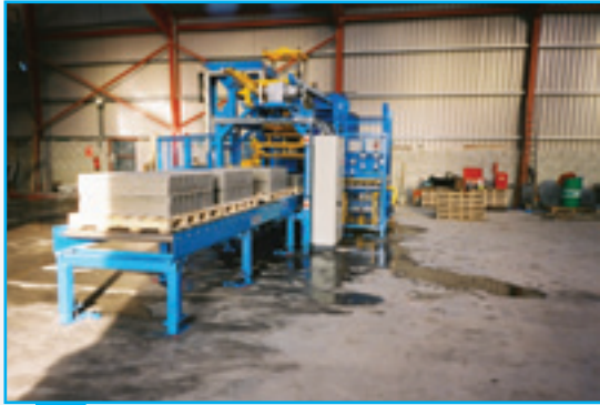
Duplex kerb production
